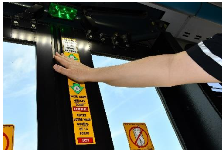
Waving your hand close to the middle of the door to open it
